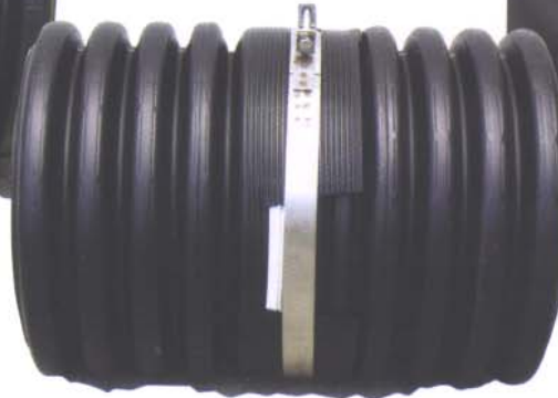
CPP 30" to 48" Meet 10.8 psi Lab Test With One ASTM-F-477 "O" Ring and a Stainless Steel Strap
